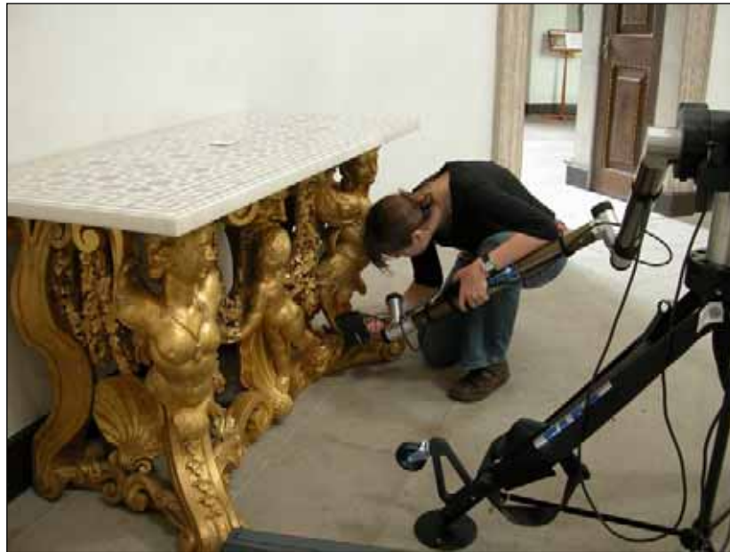
Figure 3. Laser scanning in progress.
