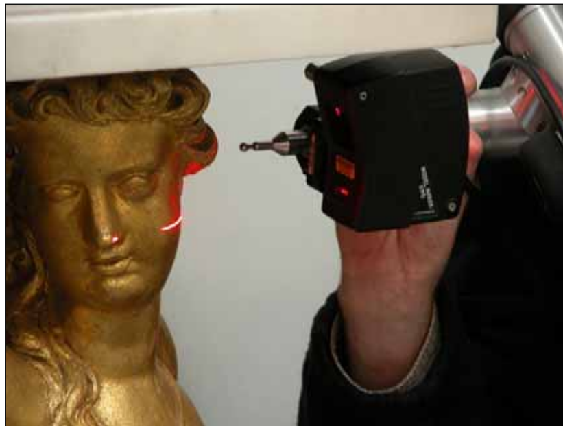
Figure 4. Detail showing sensor and laser stripe.
