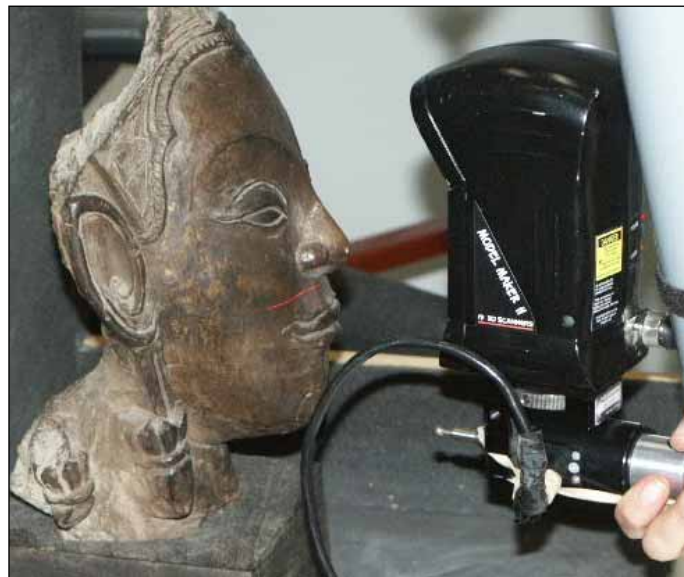
Figure 15. Laser scanning with the old 3D Scanners Modelmaker H system, used for the Chiswick tables test in 1999.
