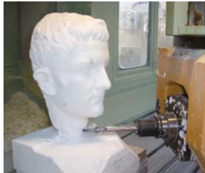
Computer - controlled machining of Caligula replica
